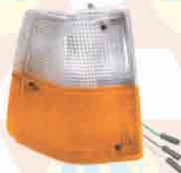
RN 9006ACR Lanterna Pisca Diant. Acrilica Bicolor Mod.Original p/ Volvo NL 10/12, L.D. N° Original: 8.121.102
